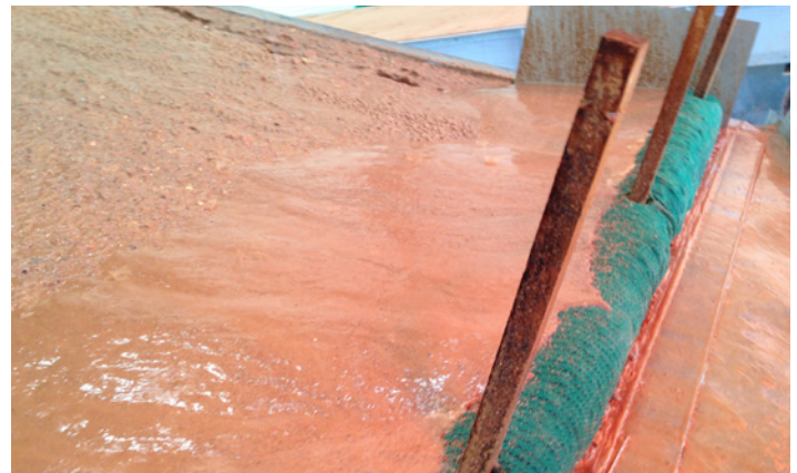
Scientific testing shows 5-inch SiltSoxx has a sediment removal rate of 95% during a 2-inch rainfall.
