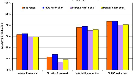
Experiment I - comparison of silt fence and three filter socks with varying physical properties
