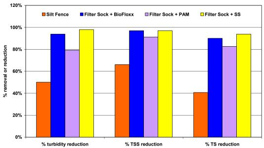
Experiment III addition of Flocculents to Filter Socks
