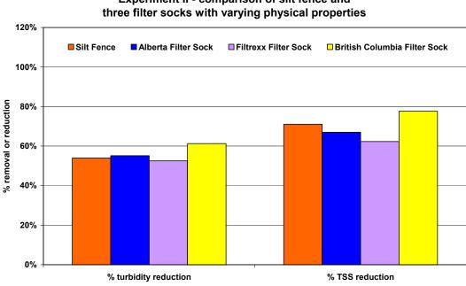
Experiment II - comparison of silt fence and
