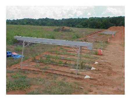
Figure 1.4: Experimental site layout with rainfall simulator.
