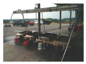
**Figure 1.1.** Rainfall Simulator and Experimental Setup.
