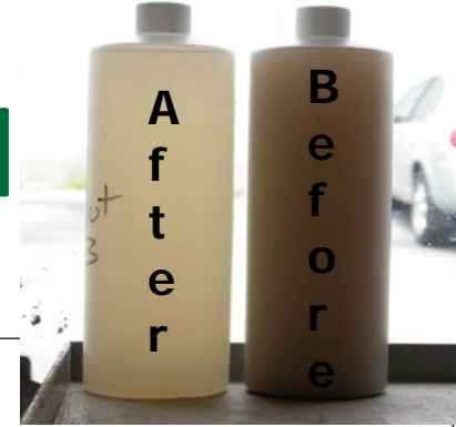
FilterSoxx Fine Sediment Removal over 30 min Runoff Event
